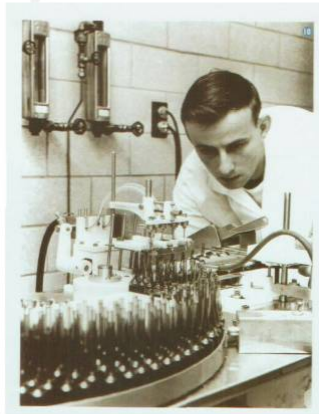
Operator adjusts machine that automatically fills and heat seals ampouls, 1957. Courtesy of the American Institute of the History of Pharmacy
